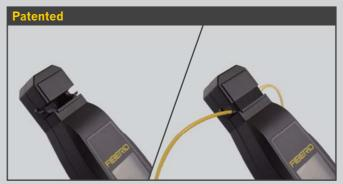
• When user pull down the trigger of FIBERID, the shielding design is able to diminish light leakage, and maintain the power value accuracy.
